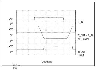
Figure 8. MAX3237 Loopback Test Result at 1000kbps (MBAUD = VCC)
