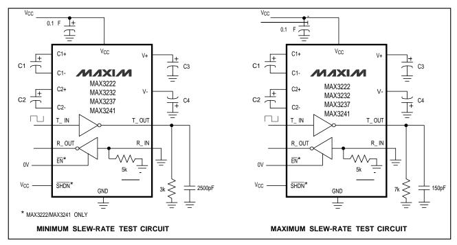
Figure 1. Slew-Rate Test Circuits
