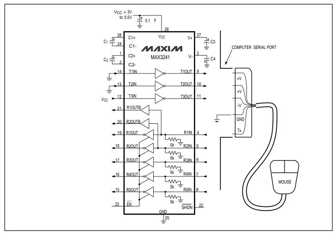
Figure 4b. Mouse Driver Test Circuit
