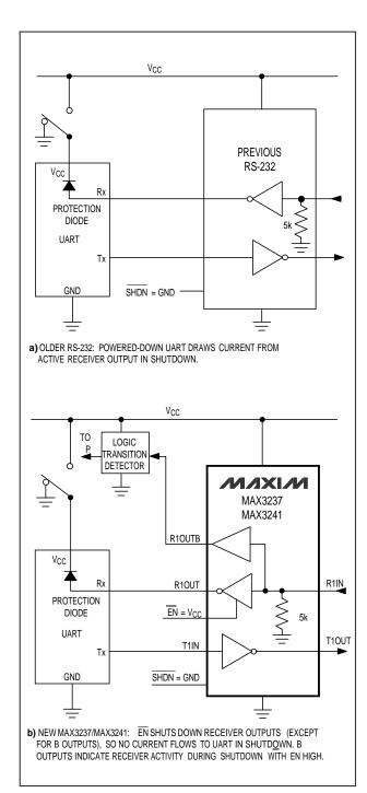
Figure 2. Detection of RS-232 Activity when the UART and Interface are Shut Down; Comparison of MAX3237/MAX3241 (b) with Previous Transceivers (a).
