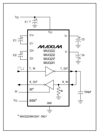
Figure 5. Loopback Test Circuit
